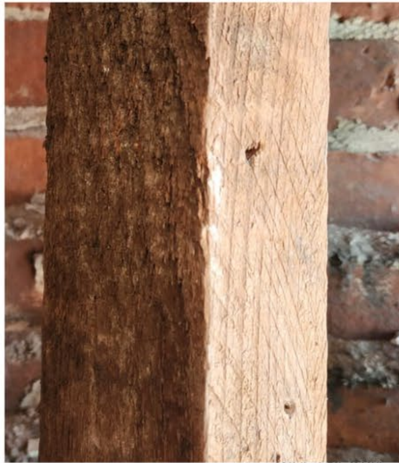
Rough Sawn on 4 sides Old Growth Douglas Fir pre 1920's Large Dimension - 2"x4"
