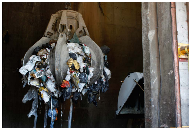
Garbage claw at the Waste-to-Energy Facility
