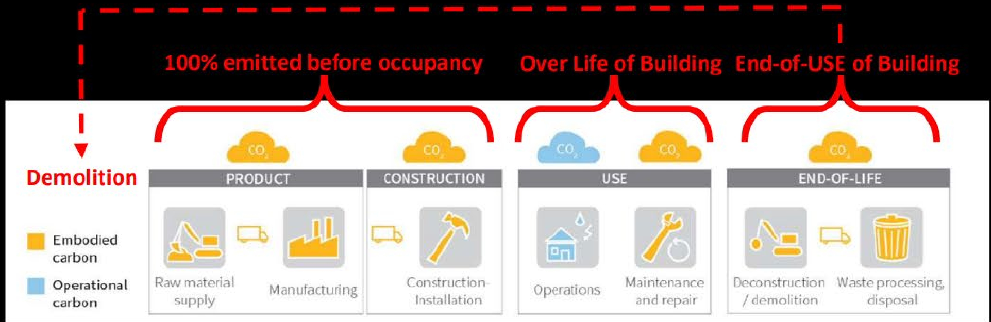
Embodied carbon and operational carbon across the key life stages of a building. CLF
