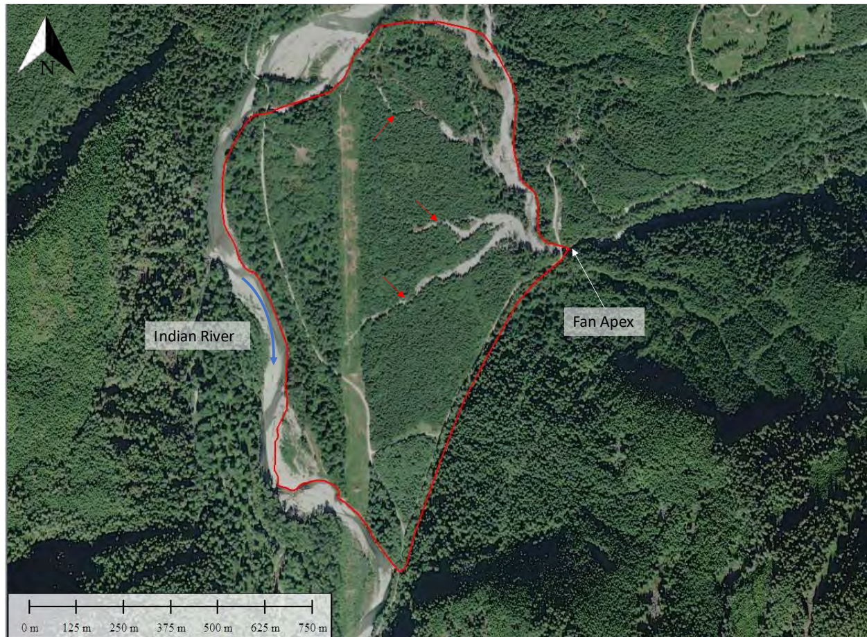
Figure B-13 Example of high evidence for previous avulsion on Hixon Creek, located North of Indian Arm. The approximate fan boundary is shown as a red polygon and avulsions are noted by red arrows.
