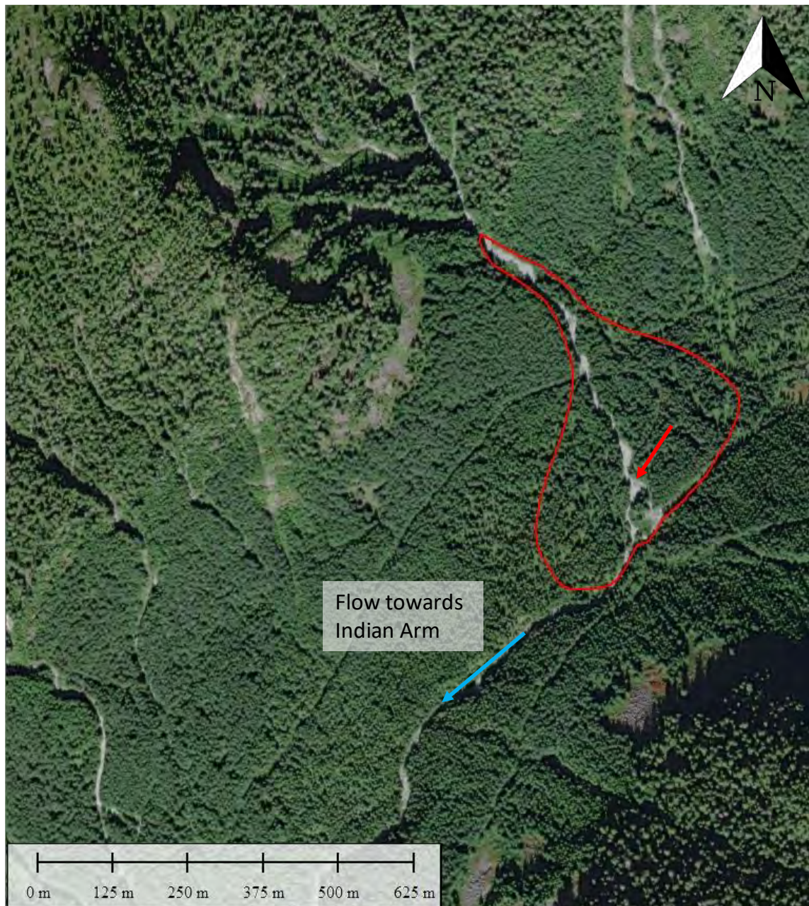
Figure B-11 Example of evidence (red arrows) for a recent debris-flow deposit on Unnamed Creek 31912, located in the east portion of the Indian Arm section of the study area. The approximate alluvial fan boundary is shown in red.
