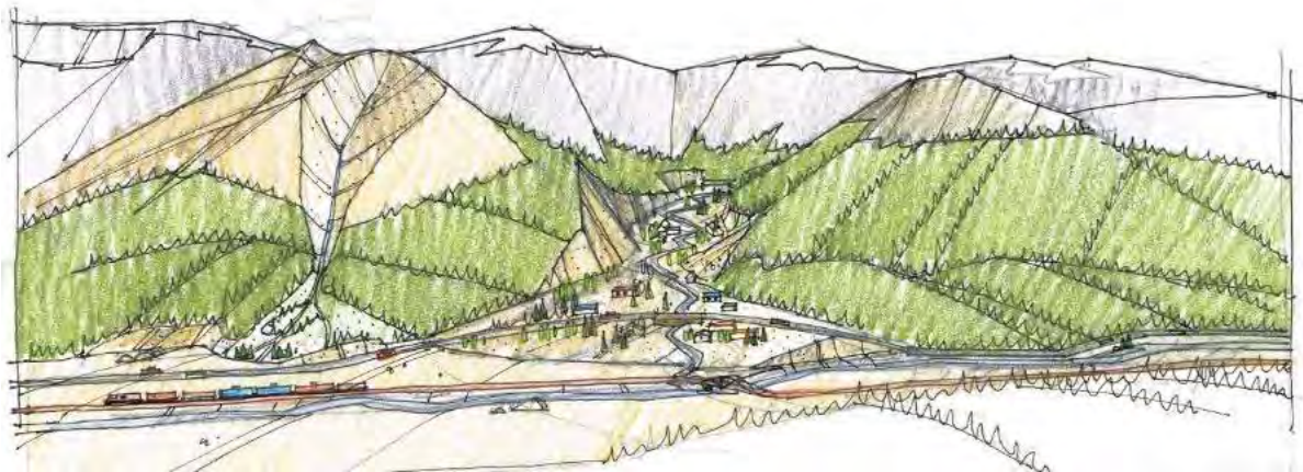
Figure B-4 Typical steep and low-gradient fans feeding into a broader floodplain. On the left a small watershed prone to debris flows has created a steep fan that may also be subject to rock fall processes. On the right a larger watershed prone to debris floods has created a lower gradient fan. Development and infrastructure are shown to illustrate their interaction with steep creek geohazard events. Artwork: Derrill Shuttleworth.
