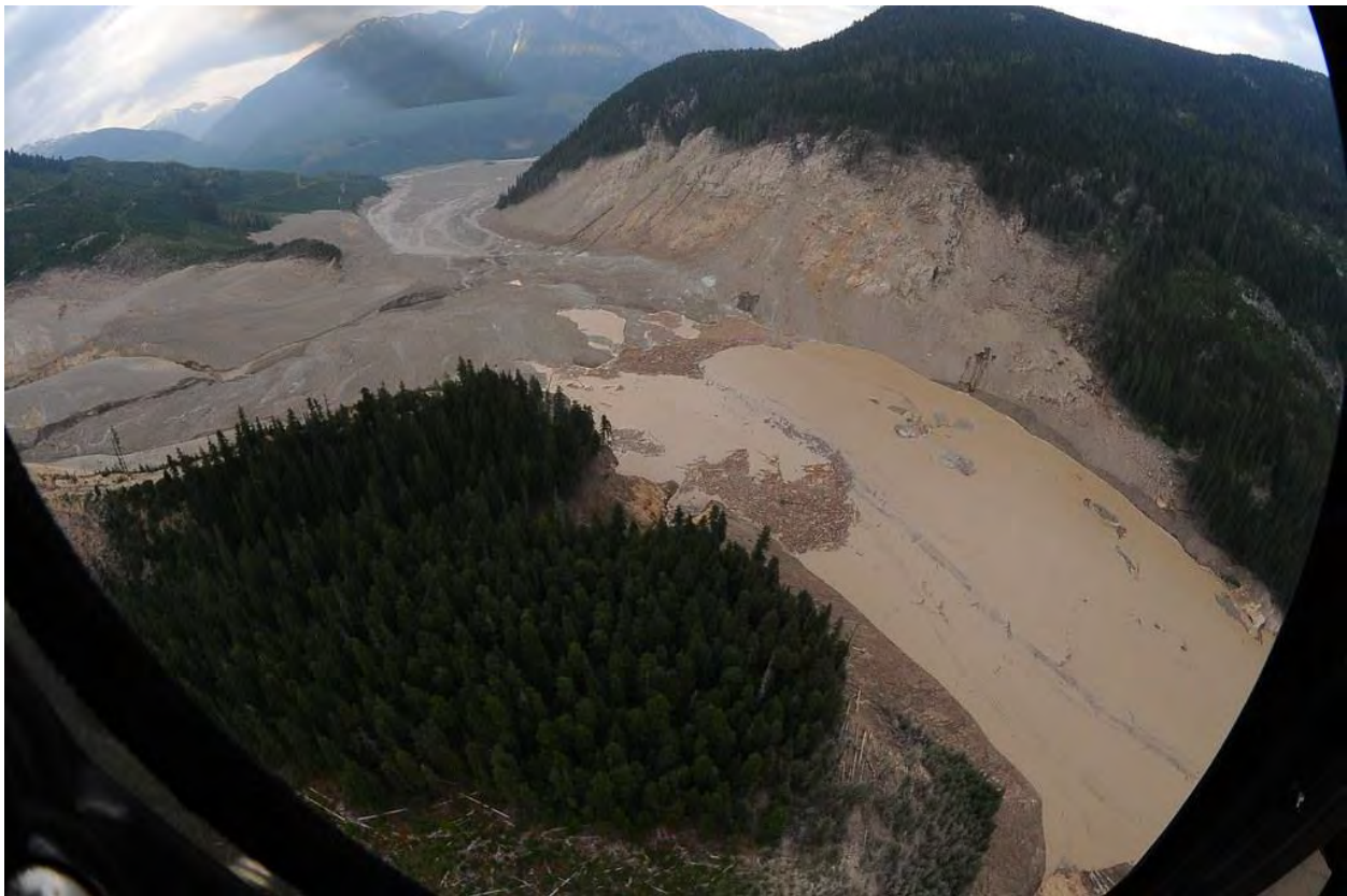
Figure B-14 Landslide dam on Meager Creek from the August 6, 2010 rockslide-debris flow from Capricorn Creek. The dam impounded Meager Creek for some time. Photo by D. Steers.
