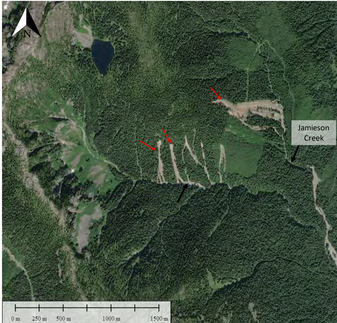
Figure B-10 Example of evidence for recent landslide or in-channel debris-flow initiation (red arrows) within the basin of Aaron and Jamieson Creek, located approximately 3.5 km west of the Indian Arm section of the study area.
