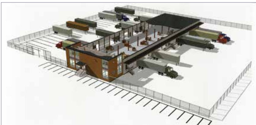
Graphic of typical freight forwarding truck terminal showing significant space required for truck loading, manoeuvring and parking.
