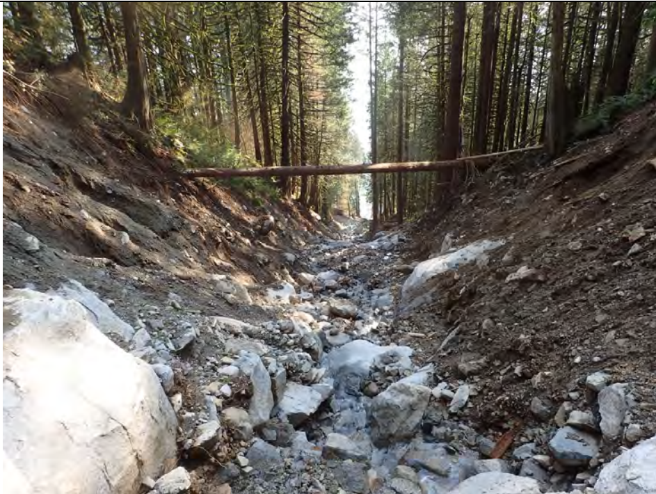
Photo 15. WP41. Note thick till deposits. Assume 0.25-1 m scour across scoured perimeter.
