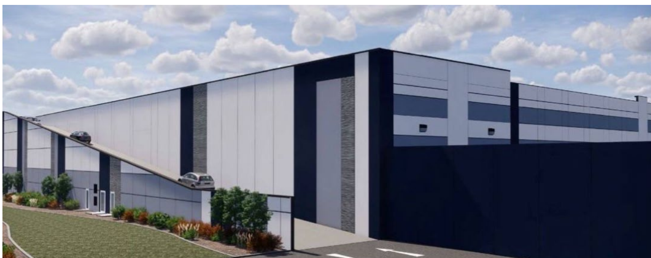
Eagle Builders' upcoming development at 3733 192 Street will be the first large-format project in Campbell Heights to include rooftop parking as an effort to create more leasable floor area than a traditional development.
