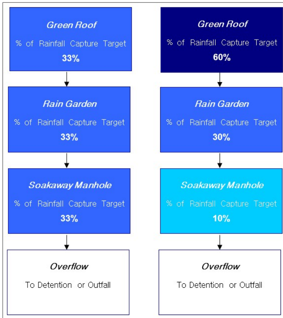
Figure 1-B: Alternative Stormwater Treatment Train for High Density Development
