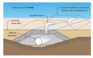
and to protect these ports from damage, the diffuser design will include a structure to deflect objects over the risers.
