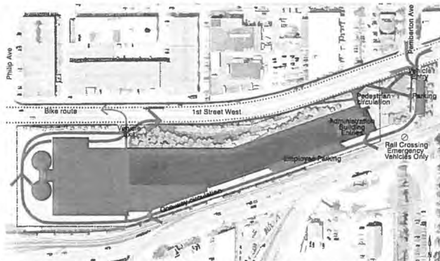
Plant circulation will be one-way with vehicles entering to the east at Pemberton Ave and exiting to the west onto 1st St
