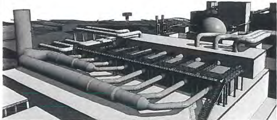
The treated air at the top of the biotowers will be discharged to activated carbon units for final polishing.
