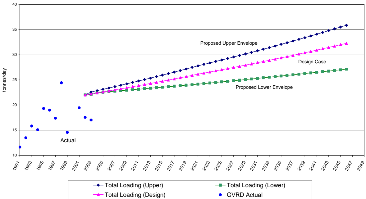
FIGURE 3.7 LIONS GATE WWTP GRAPH OF THE LOWER, UPPER ENVELOPE, AND THE DESIGN CASE SCENARIO FOR TSS (MAX. MONTH)
