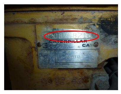
The engine serial number data plate from a 1992 Caterpillar 14G motor grader. The serial number reads 08Z68216
