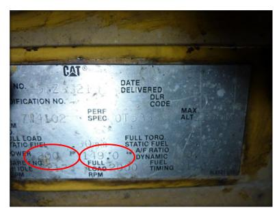
This engine data tag from a 1992 Caterpillar 14G motor grader shows the engine power rating is 200 hp or 149 kW.
