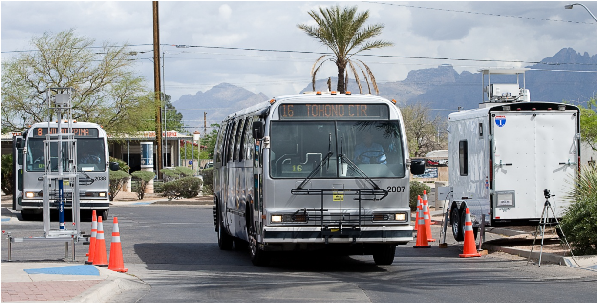
Figure II-2: Example On-road set-up of RSD for High Tailpipe Transit Bus
