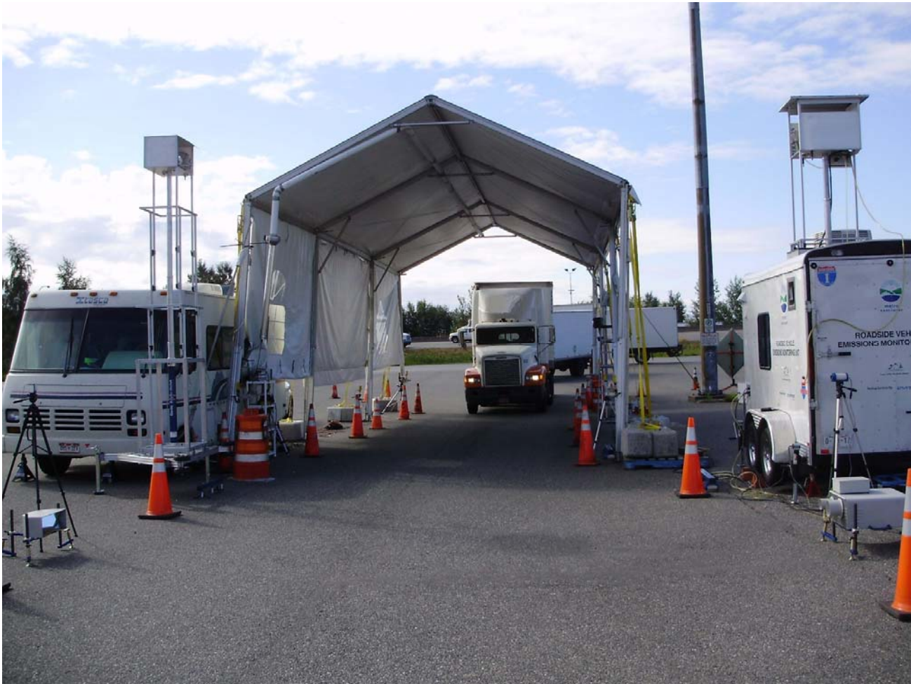
Figure II-6: HDET Test Tunnel
