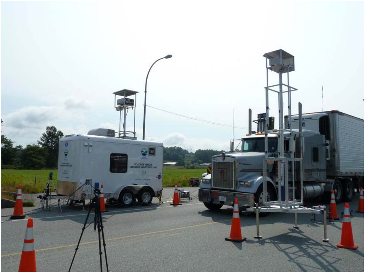
Figure II-3: On-road set-up of RSD for a High or Low Tailpipe Vehicle
