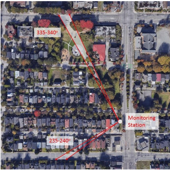
Figure 6.9: Two five-degree wind sectors representing differing distances to a major roadway.
