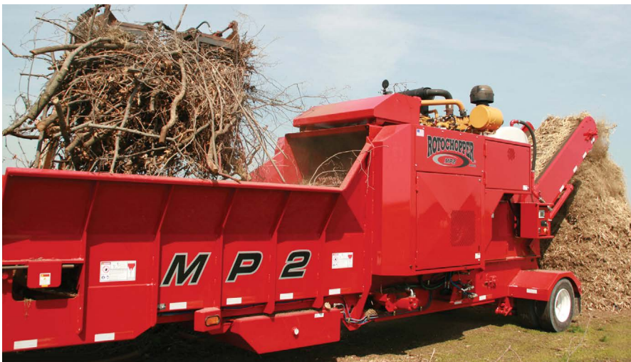
Figure 4. Large tub grinder for clearing land and orchards. Photo credit: P. Doig.
