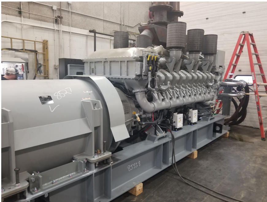
Factory Testing of one Genset
