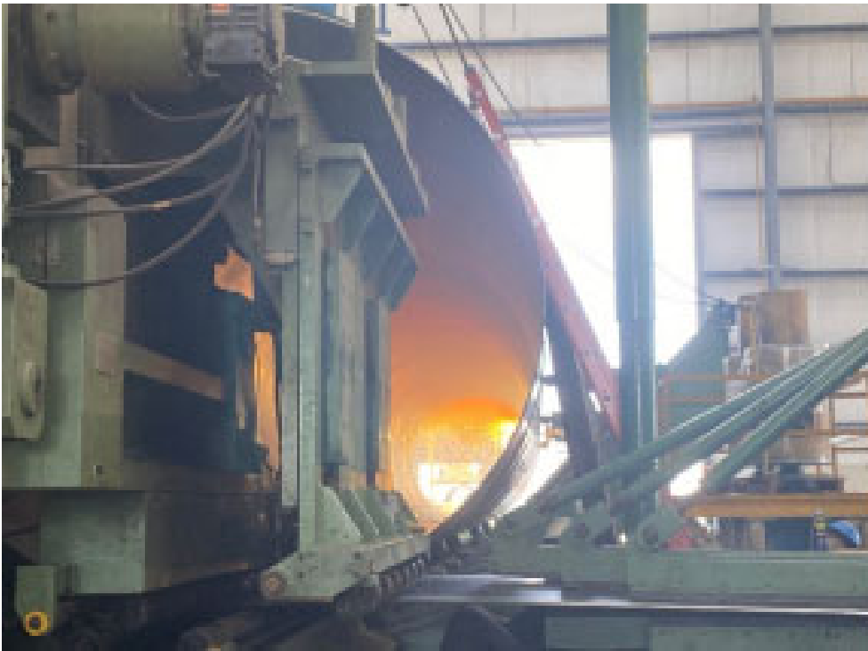
3.2 m Diameter steel pipe in production
