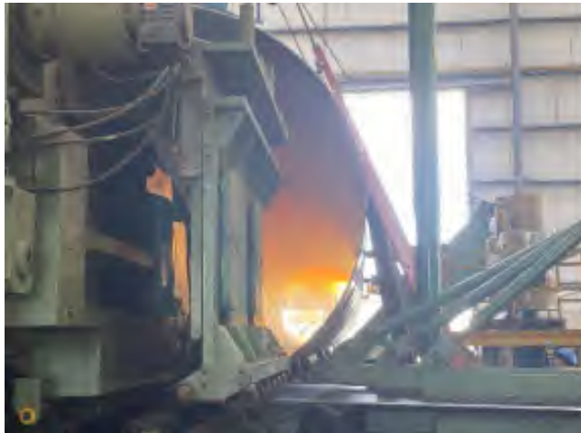
3.2m Diameter steel pipe in production
