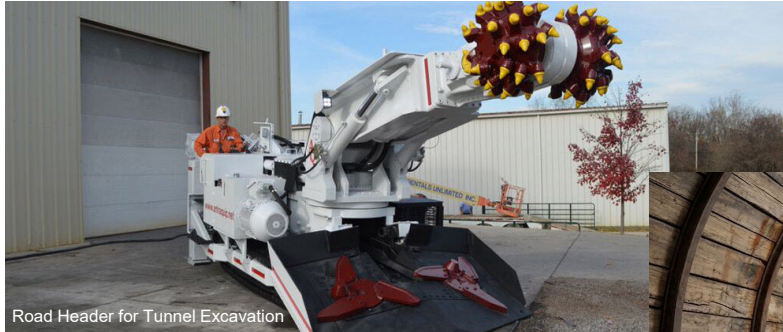
Road Header for Tunnel Excavation
