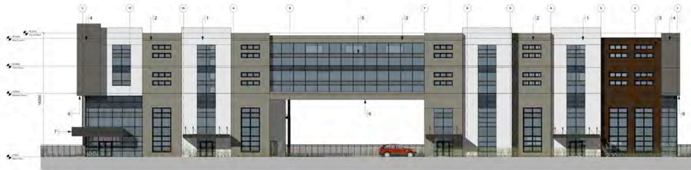
2 NORTH ELEVATION (64 AVE) Scale: 1:150
