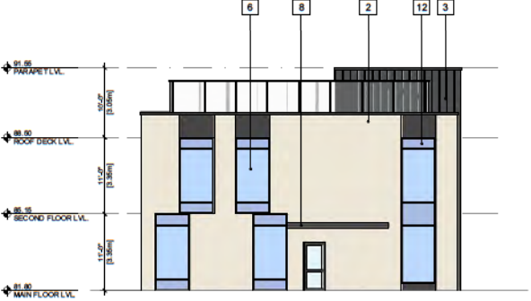
4 BUILDING-2 WEST ELEVATION Scale: 1/16"=1'-0"
