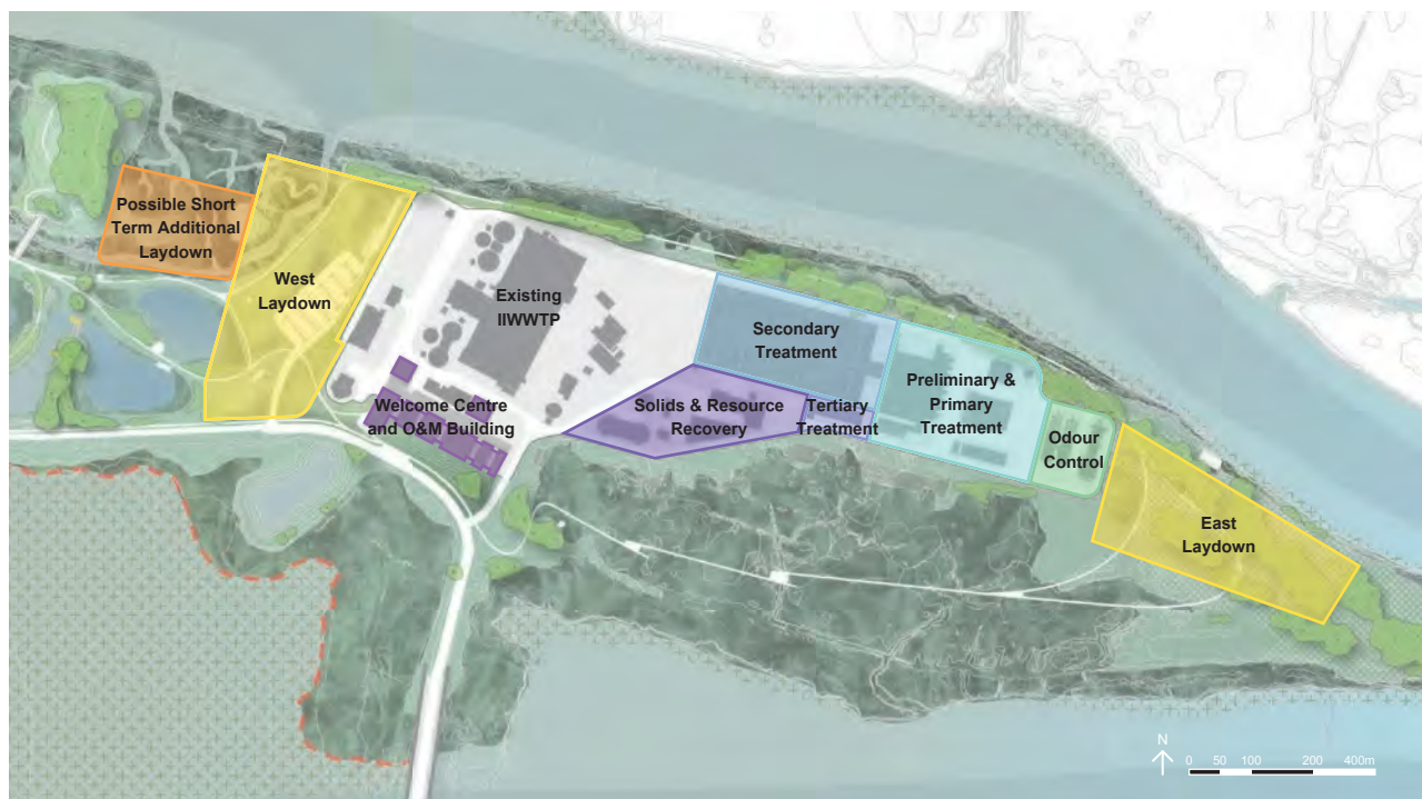
Figure 25. Diagram depicting peak laydown requirements for the construction of the IIWWTP Projects. **NOTE: Drawings as shown are conceptual and subject to additional study and design development.
