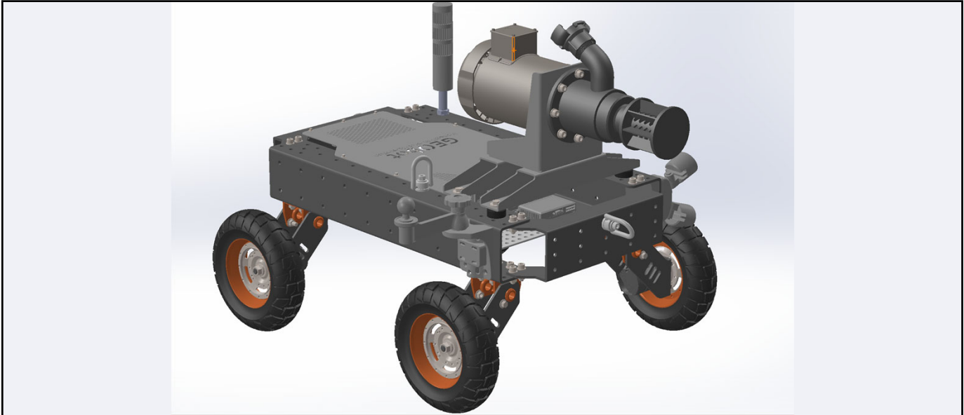
Rendering of robotic sprayer for Multi-Composite Coating. Image courtesy of UBC.
