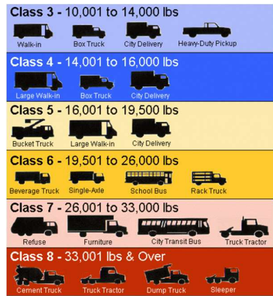
Image Source: Examples of Trucks adapted from Fact #707: December 26, 2011 Illustration of Truck Classes Vehicle Technologies Office
